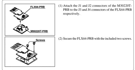
Figure 3.3 Connecting the M30220T-PRB pod probe
